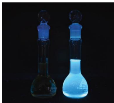
Figure 1.7. A visual illustration of the large fluorescence enhancement of a guest molecule which can be obtained by CD-host inclusion: the fluorescence of a 5.0 \times 10^{-4} M solution of 1,8-ANS under UV-A irradiation in the absence (left) and presence (right) of 20 mM HP- \beta -CD.
